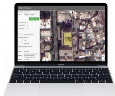
Use the Sun Analyzer Tool, **Simulate** the shadows on roof for any day of the year and record impact of shading caused by parapet walls, water tanks, exhaust vents, panel shading, trees, etc.
