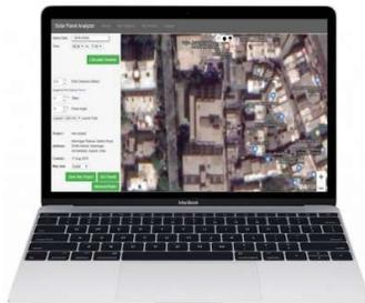
With **Google Map Interface**, draw line, polygons or any shape for a simple modeling and creating a roof plan for work area & shadow objects like parapet walls, water tanks, exhaust vents, panel shading, trees, etc.
